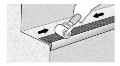
Once in place, roll over the Insert to ensure consistent adhesion and a secure bond. Please take care not to stretch the Insert when rolling. Leave for a few hours to ensure proper bonding.
