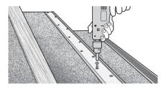
If installing on a concrete substrate, lay cut profile on the stair edge in place then mark the c/sunk holes with a marker then remove profile. Using a 5.5mm masonry drill bit on a drill with hammer function, gently drill the holes on the marks to a depth of 35mm max. Once complete, clean holes from concrete dust and tap the nylon plugs into holes ensuring the are recessed slightly. Reposition the profile and screw the profile down fastening it tightly.
