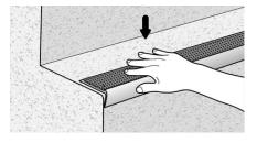
Install by placing the Insert into the nosing and pressing into place without undue stretching.
