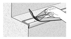
Remove the adhesive backing liner from the Tredsafe Insert.
