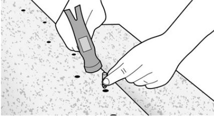
Clean away the concrete dust from drilling and push in by hand or lightly tap the plugs into the holes with a hammer.
