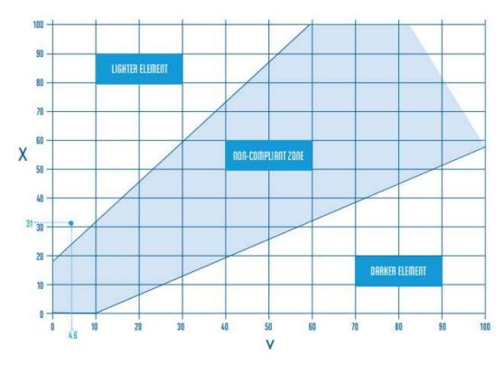
NOTE: Luminous reflectance of building elements must lie outside the shaded area. Of the 2 elements the lighter element is to be above the shaded area and the darker element is to be below the shade area
